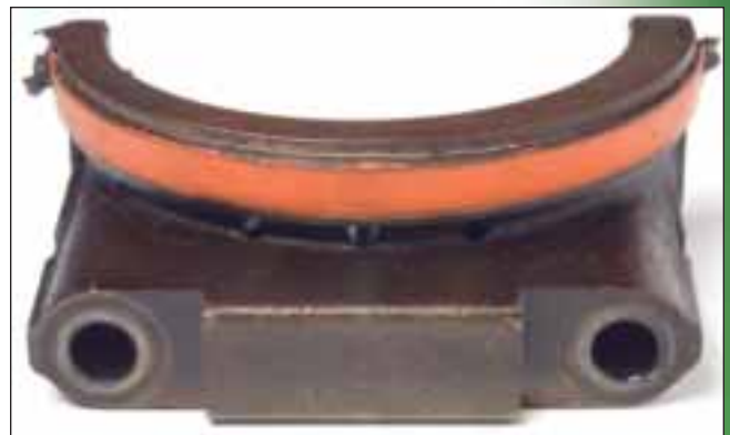
The rear main bearing cap and oil seal were in good condition. The rear seal was very pliable and still intact, showing no signs of deterioration.
